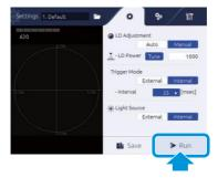
The measurement screen is displayed, and a measurement with the changed content is performed.
