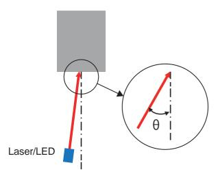
With an internal light source, the angle of  $2\theta$  is measured and the value of  $\theta$  shown through calculation. With an external light source, the value of  $\theta$  is shown as is.
