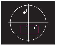
Target: Spot-1→OK Target: Spot-2→OK Target: Spot-3→NG
