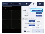
4 Set the number of measurement spots with [Max Spot Number], and set the judgment target spot with [Target].
